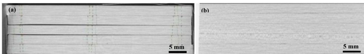
**Figure 3.** CT-slices of mounted CFRP-plates: In (a) air gaps are visible, in (b) air gaps are almost completely removed by using a plastic interlayer and applying a proper mounting.
