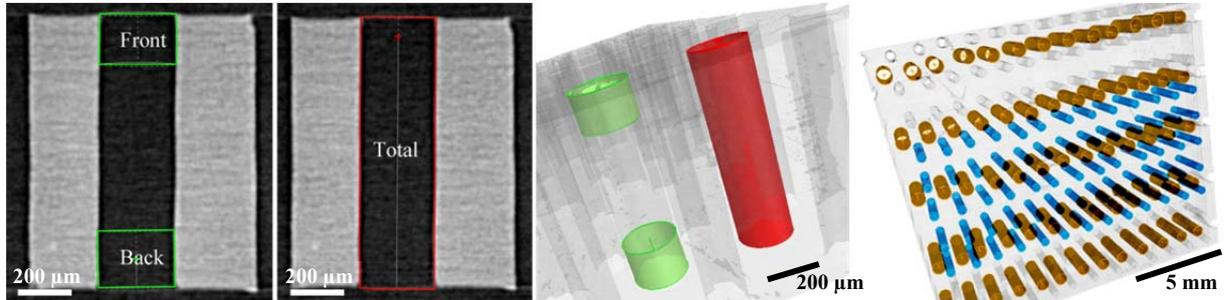
**Figure 6.** Cylinder fit within the CT-data of drill hole, front/ back (green) and total (red) to obtain the diameter of the drill holes accurately. All 65 fitted cylinders of Sample D3 are shown in the right figure, in orange 0.3 mm and in blue 0.2 mm holes. The voxel size of the CT-measurement was  $(5 \mu\text{m})^3$ .
