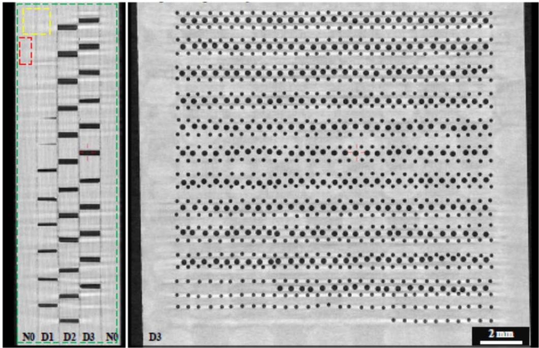
**Figure 7.** CT-slice images of combination S3 of different plates (N0 - D1 - D2 - D3 – N0) to create a porosity reference sample with an expected porosity of 4.81 vol. % (Adapted from ref. [5]).
