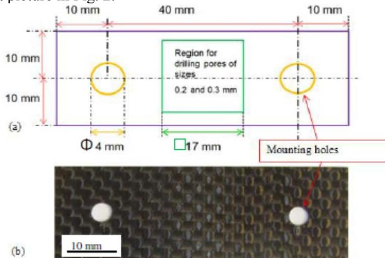
**Figure 1.** Schematic of dimensions of the drilled CFRP plates (a) and photographic picture of a typical CFRP-plate (b). The thicknesses of the CFRP plates are around 1 mm. The drilled CFRP-plates were mounted together by screwing from the front and back side through the mounting holes.
