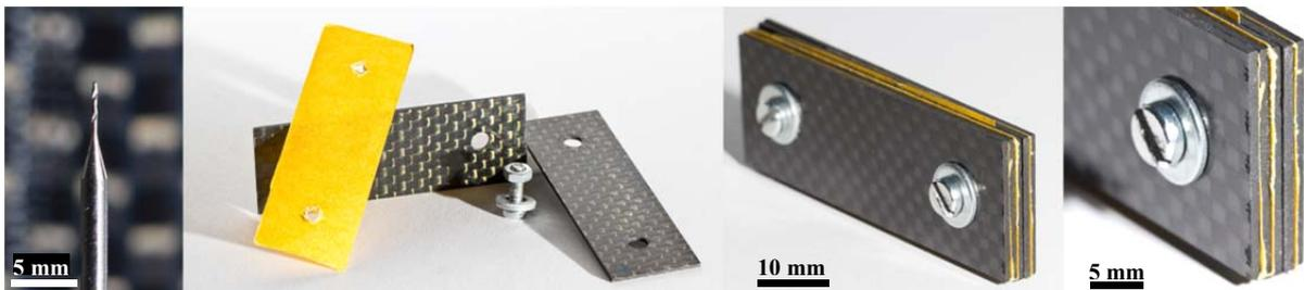
**Figure 2.** Overview of fabrication the reference porosity samples. Artificial holes were fabricated by micro-drilling (left picture). Three drilled CFRP-plates were mounted together by screwing from the front and back side (right picture).
