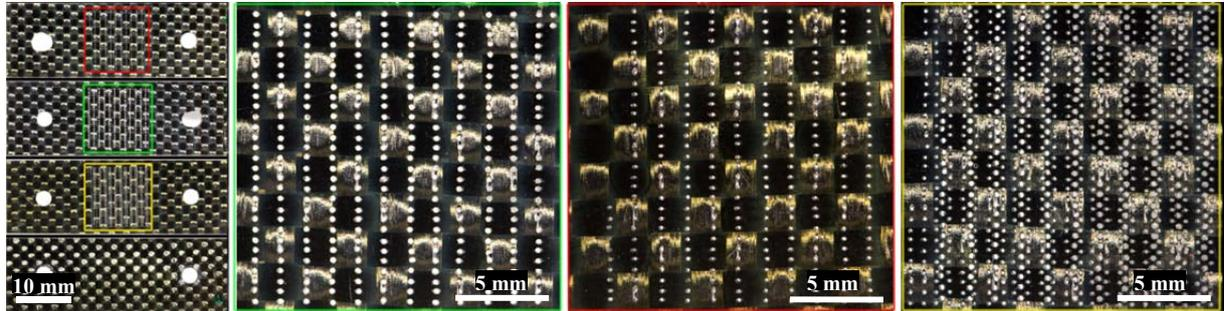
**Figure 4.** Overview of drilled and undrilled plates (left) and three samples containing different number of drill holes with different diameters. Detail of the sample D2 with 0.3 mm drill holes (green), detail of the sample D1 with 0.2 mm drill holes (red) and detail of samples D3 with 0.2 mm and 0.3 mm drill holes (yellow).
