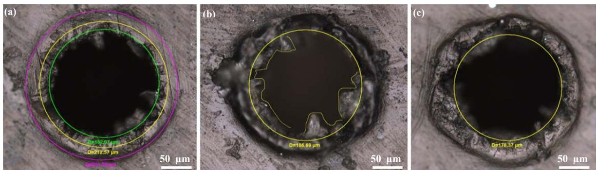
**Figure 5.** Delamination visualised under microscope (a) area of impact (b) ingrowth of CFRP in void region (c) outgrowth of CFRP around drilled region.
